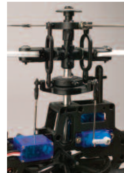
The composite 120 degree CCPM swashplate is very rigid and robust for better control.
