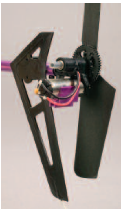
The N-60 Heavy Duty tail motor is larger than the N-30 found on most helis.
